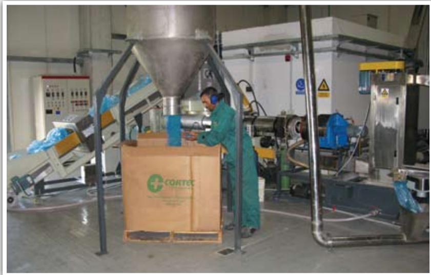
In-house recycling is performed in EcoCortec plant using modern top quality reprocessing line
