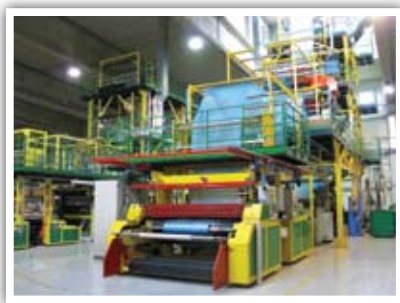
State of the art extrusion line in EcoCortec plant especially designed for high tech VpCI 126 films.
