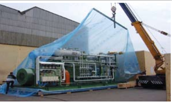
VpCI-126 Blue films and bags protect metal objects as small as a needle, to as large as the contents of an oceangoing container as shown in picture
