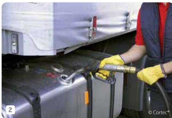
2 Adding VpCI®-706 to diesel tanks before shipment or storage prevents the formation of corrosion.
