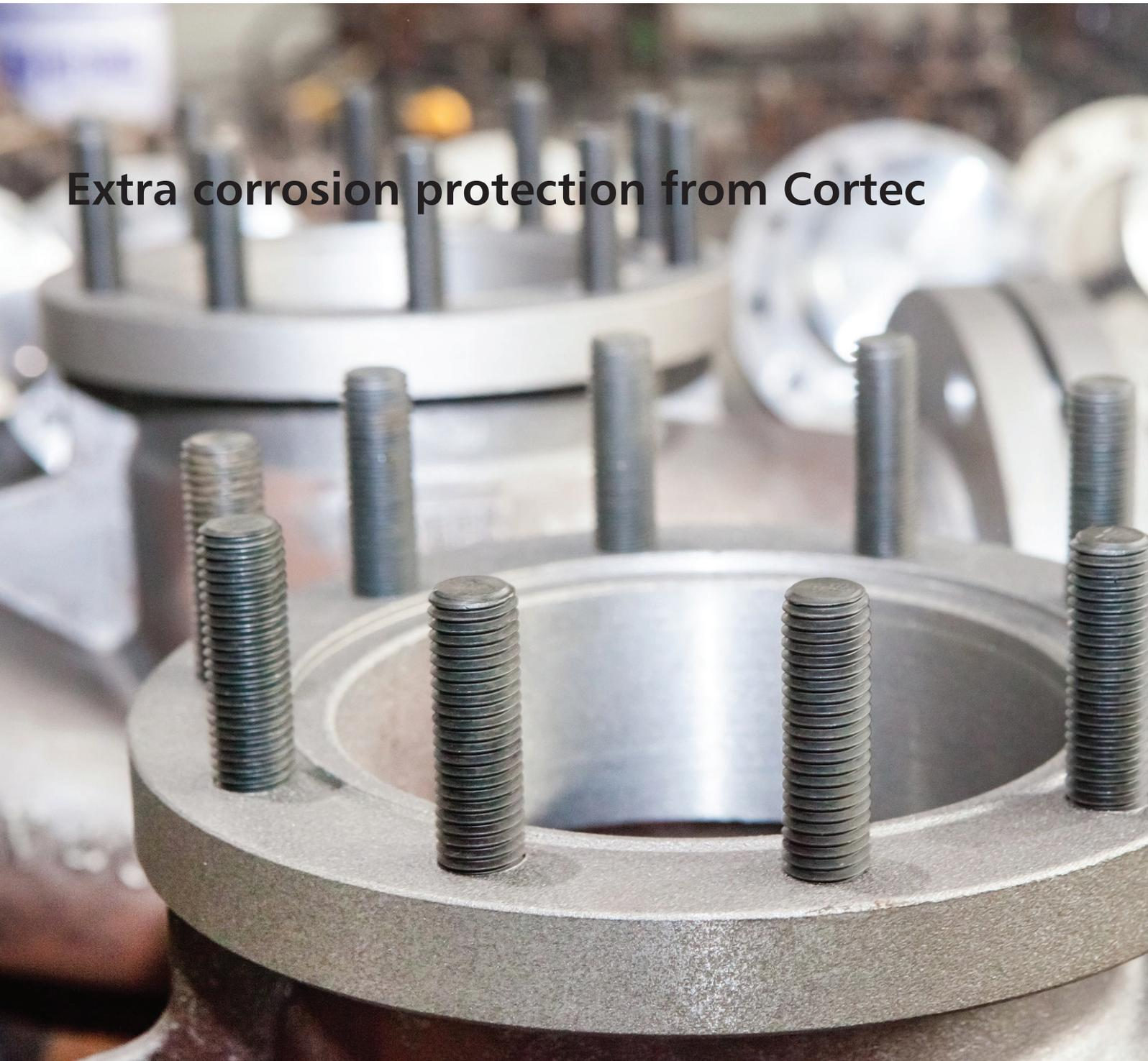
Extra Vapor phase corrosion inhibitors have been added to Cortec's VpCI-368 coating for added protection.
