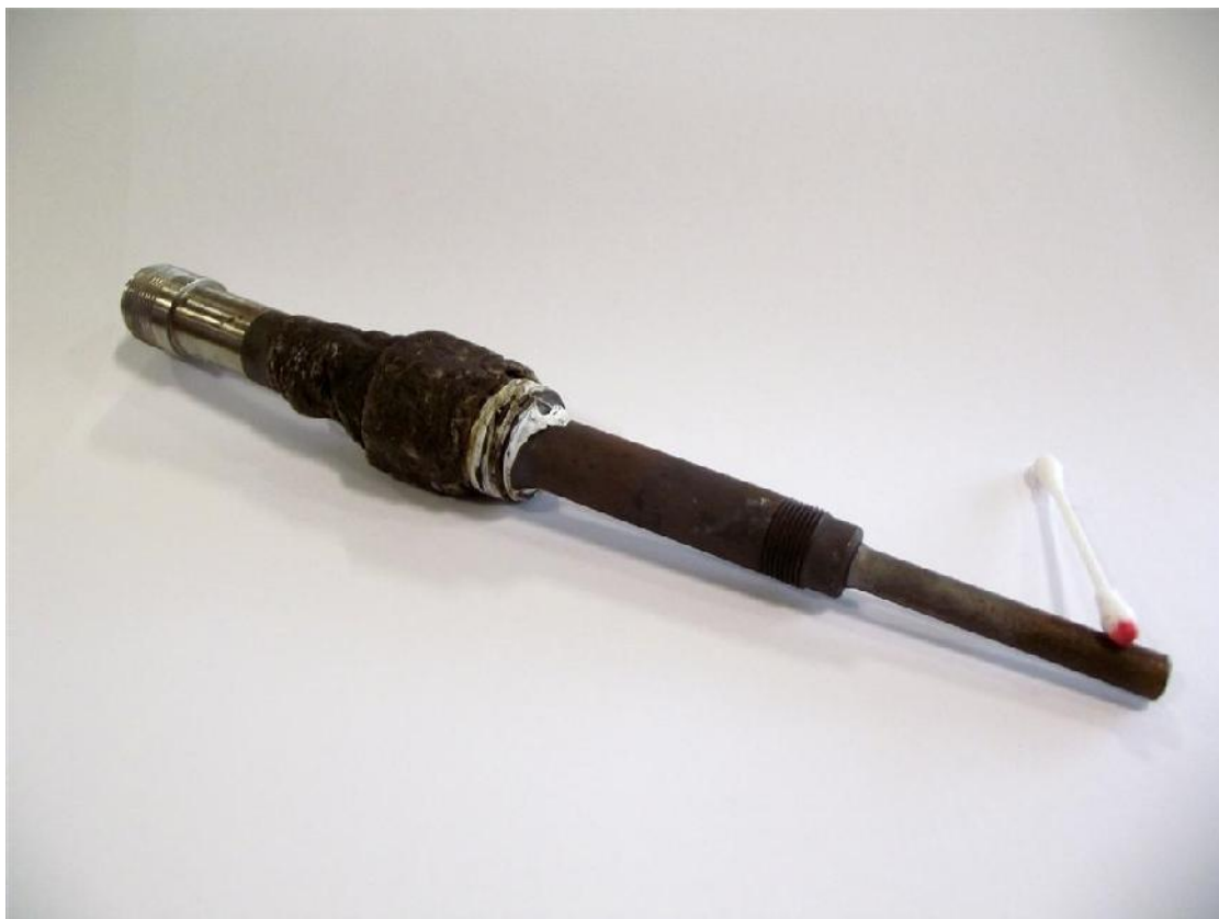
Figure 5: Positive inhibitor test on the sensor end of a corrosion probe.
