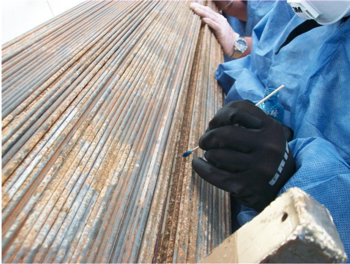
Figure 4: Swab test for inhibitor during cable inspection.
