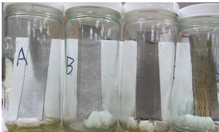
FIGURE 2 Setup of corrosion testing in a simulated hydrotesting environment.
