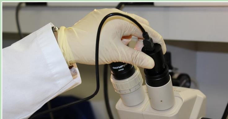
The simple addition of a camera to one of the microscope eye-pieces allows for greater precision and ease in analyzing Cortec's products.
