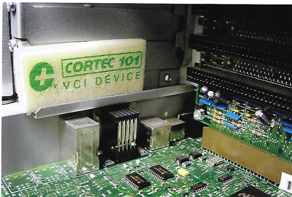
The Cortec Vapour phase Corrosion Inhibitor 101.
