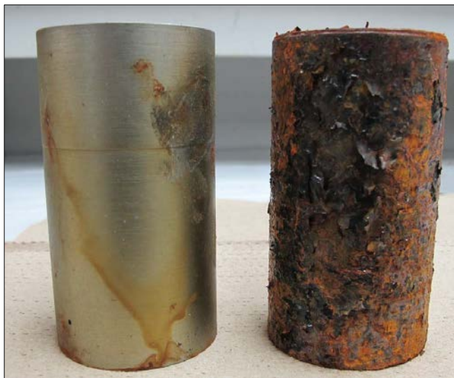
Coated pieces after 600 hours in ASTM B-117 salt fog testing; VpCI®-368 on the left, black paint on the right.
