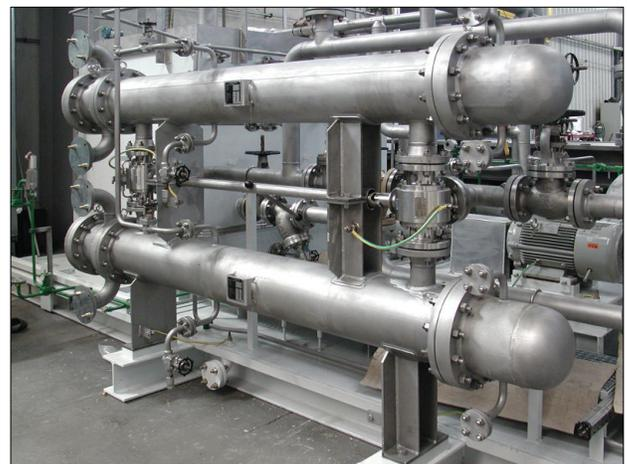
VpCI®-371 turned out to be just the high temperature coating a manufacturer of oil coolers was looking for as it tried to reduce the high cost of using stainless steel while maintaining corrosion resistance. The company manufactures hundreds of oil coolers for a major producer of heavy equipment. When carbon steel oil coolers had been used inside the heavy equipment, corrosion was found at the six-month
