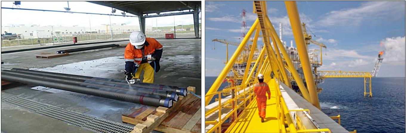
Coated materials can be protected for up to 5 years. When necessary, the VpCI<sup>®</sup>-391 coating is easily removed with alkaline cleaning. This means that large metal parts or equipment can be stored outside for extended periods of time. When needed, they are easily inspected, cleaned, and put into service. It saves on valuable warehouse space while assuring that metal parts can successfully weather through outside storage.
