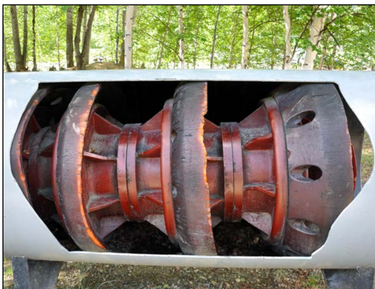
Side view example of Pigging in Pipeline.
