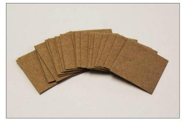
corrosion protection. The inhibiting coating does not alter the appearance of products or require removal before further finishing or use. The paper is coated on both sides for fast vaporization, excellent contact protection, and superior corrosion protection for both ferrous and non-ferrous metals.
