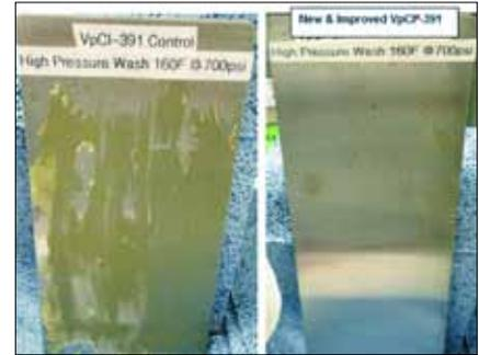
Removability of VpCI®-391 (tack free temporary coating) has been improved without affecting the current protection properties of the product. The VpCI®-391 was removed with hot (160 F°) high pressure washer at 700 psi, as seen in the panels above.
