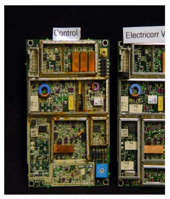
ASTM D-1748 Standard Test Method for Rust Protection by Metal Preservation in the Humidity Cabinet
