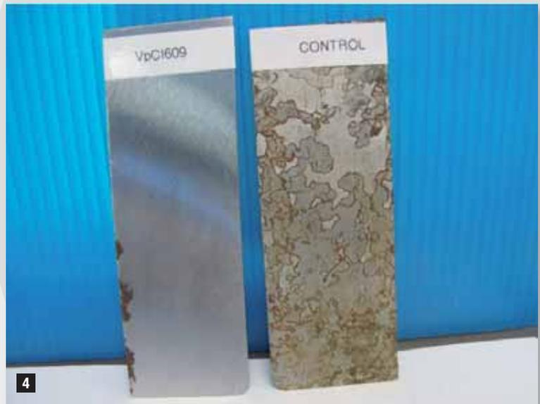
**4** *Panels after 2 weeks in sand. According to the test results VpCl®-609 provides excellent corrosion protection in the sand saturated with the submitted water sample*
