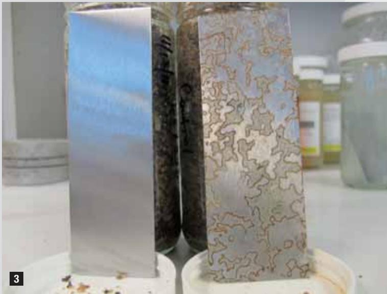
**3** *After one day. No corrosion was found on the panel from the jar with VpCl®-609 and ~ 95% of the surface of the panel was corroded in the 'Control' jar.*
