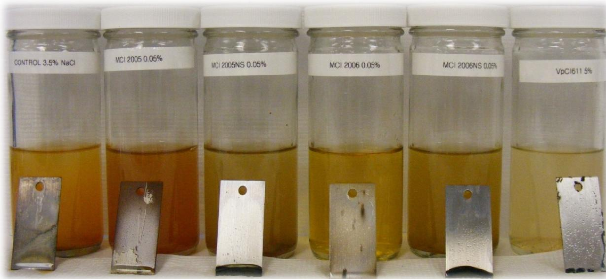
Picture 23. Carbon steel plates after 240h in 3.5% Sodium chloride solution
