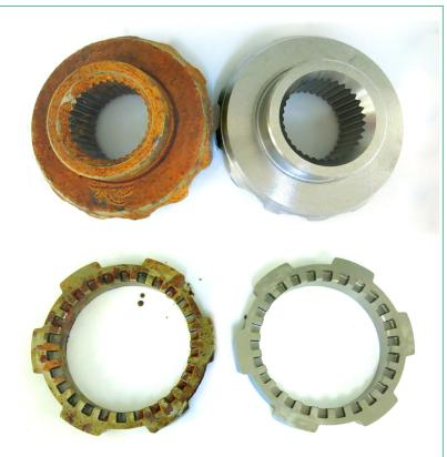
Maximize protection by overlapping Cortec® VpCl® systems: At left, unprotected sintered parts were corroding after 15 hours of ASTM D-1735 testing in a 100% relative humidity chamber at 100.4 °F (38 °C). At right, parts protected in dual system of VpCl®-146 paper inside a VpCl®-126 bag remained corrosion free after 427 hours in the same test conditions.
