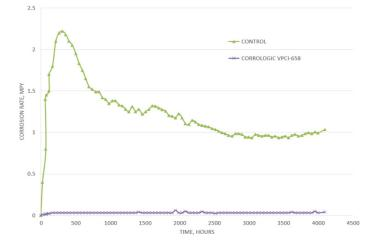
ER (electrical resistance) probe corrosion readings over 4000 hours of testing.
