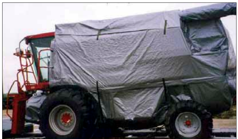
International Harvester equipment prepared for export shipment using Ecoshield® custom VpCI® covers.
