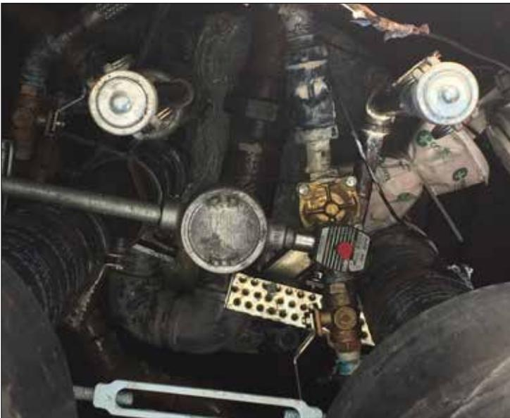
A cleaned and coated sump with a VpCI®-308 pouch tied in to saturate the space with vapor phase corrosion inhibitors for extra protection.
