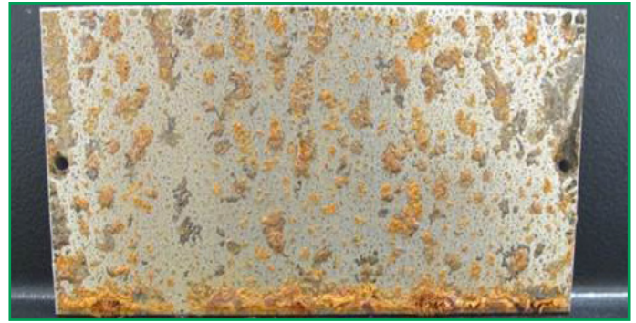
Control panel after 860 hrs in ASTM humidity test
