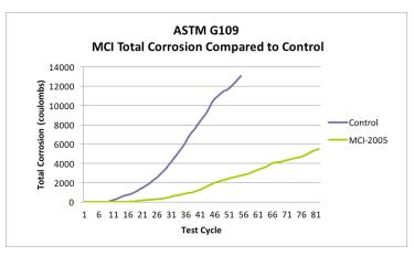
ASTM G109 - Standard Test Method for Determining Effects of Chemical Admixtures on Corrosion of Embedded Steel Reinforcement in Concrete Exposed to Chloride Environments
