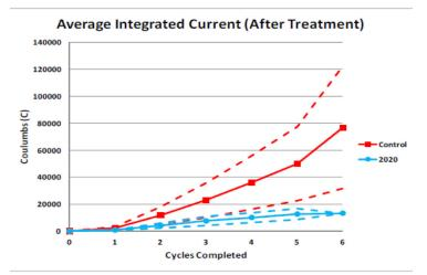
Results of the US Bureau of Reclamation M-82 (M0820000.714) Standard Protocol to Evaluate the Performance of Corrosion Mitigation Techniques in Concrete Repairs. Results are of MCI®-2020 applied under a standard sealer.
