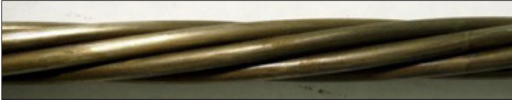
Figure 6: MCI®-309 Treated Specimen from Saltwater After Cleaning (Middle)
