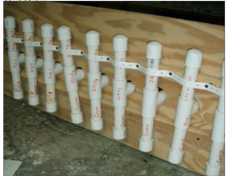
Figure 3: Corrosion Test Setup, Pennsylvania State University Grouting Laboratory Report
