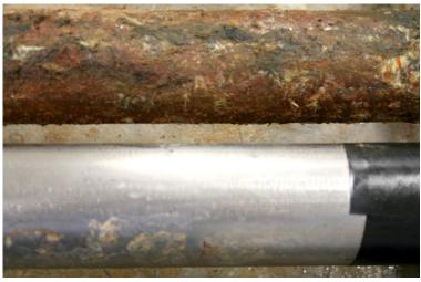
Pipe surfaces after 210 days of corrosion testing. VpCl $^{\ensuremath{\$}}$ -658 was applied to the bottom pipe.
