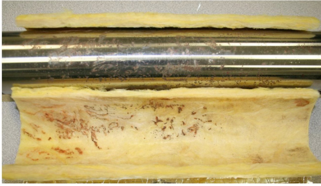
Unprotected pipe, after 240 hours of testing in high temperature conditions with regular chloride injection.
