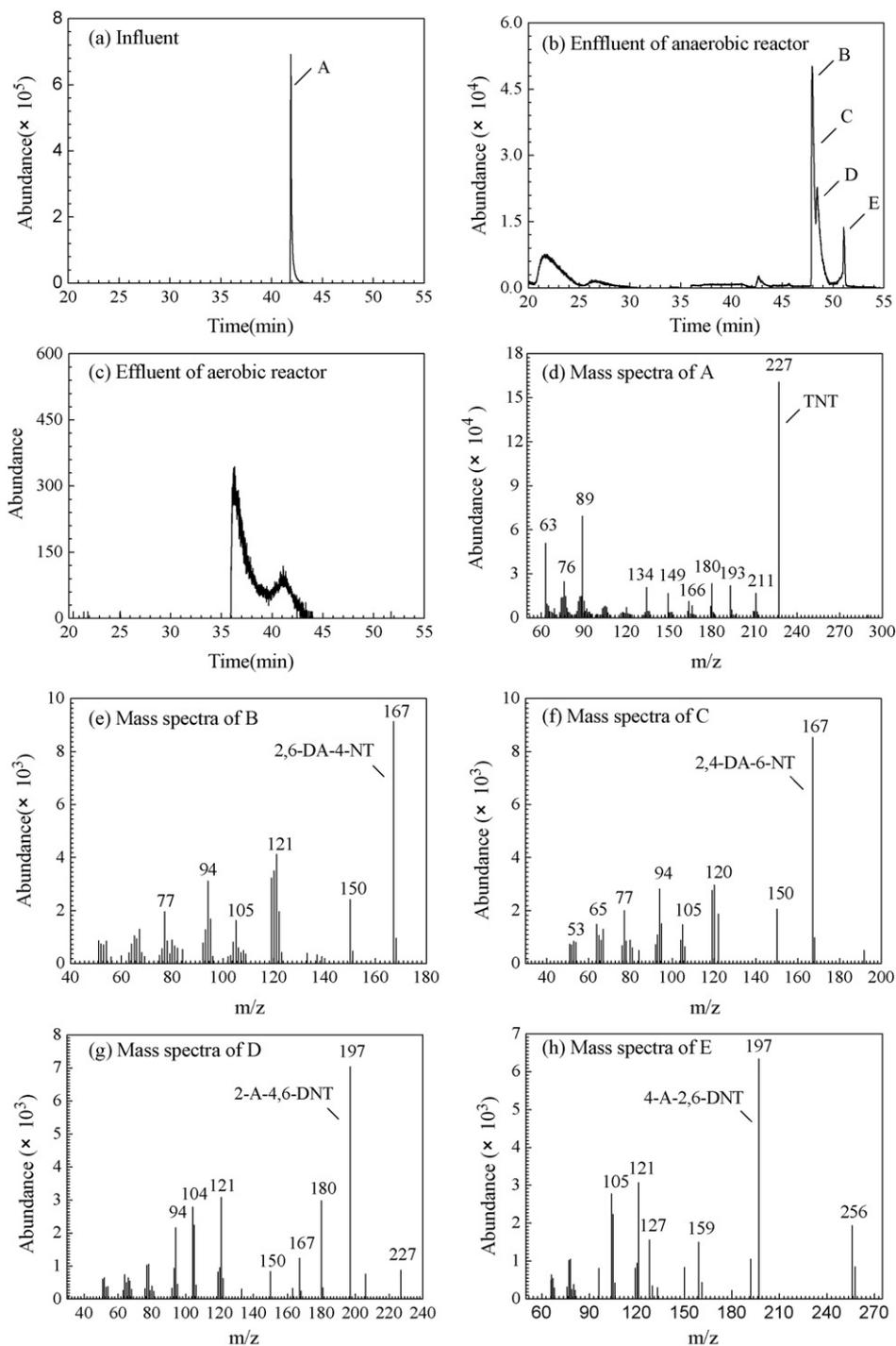
Fig. 4. Spectrum of influent and effluent organic components for anaerobic and aerobic reactors.
