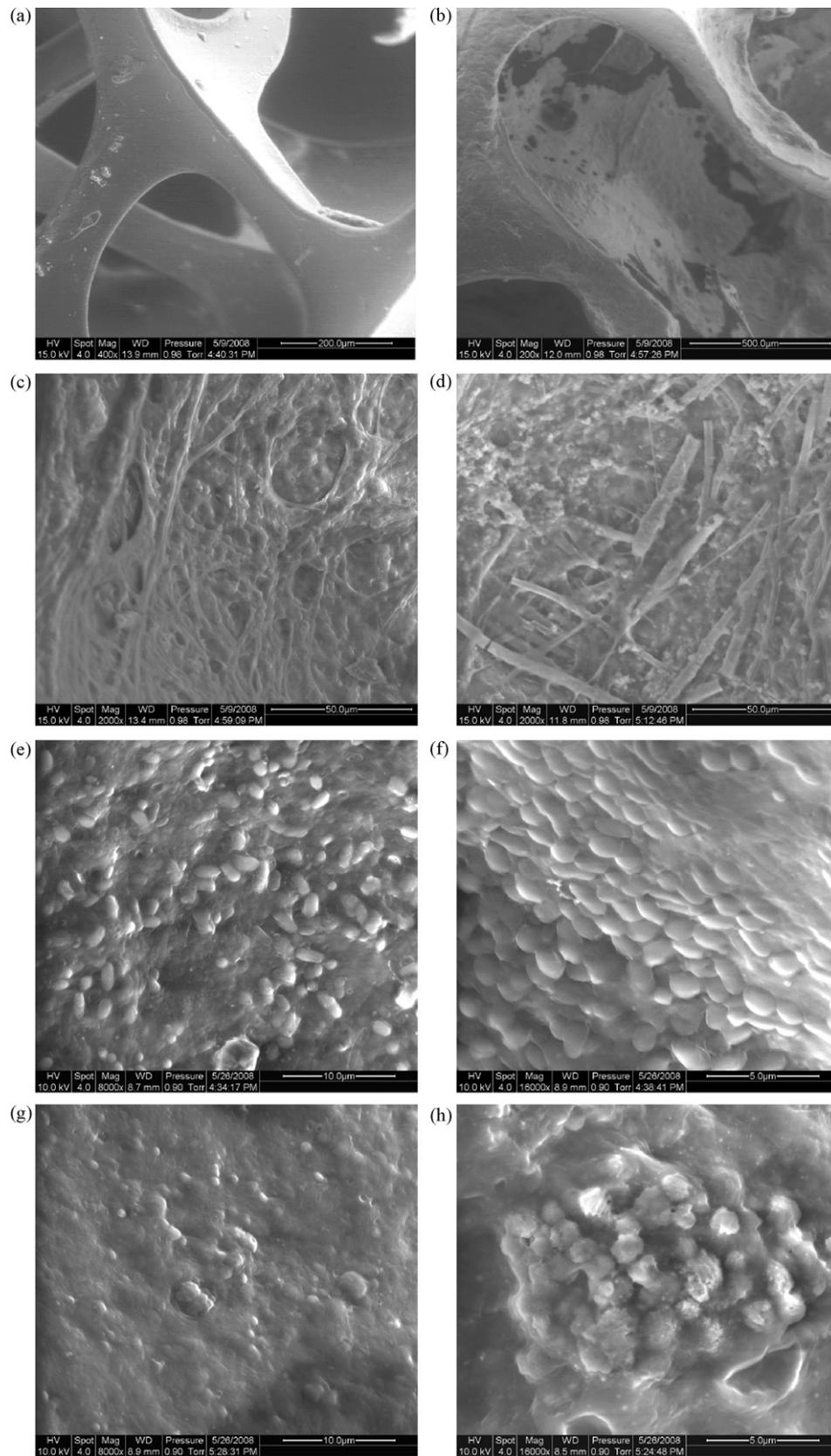
**Fig. 8.** Carrier and microorganisms observed in reactor by ESEM.
