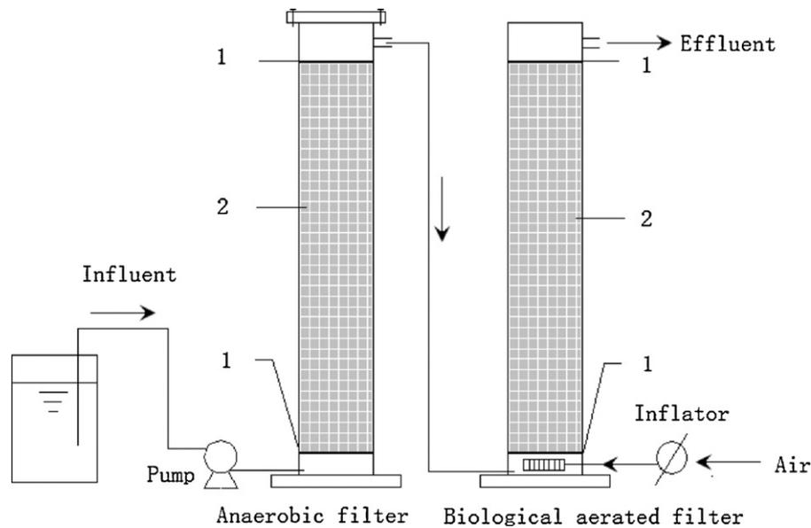
Fig. 1. Reactor system: (1) clapboard, (2) carrier and microorganisms.
