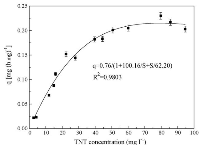
Fig. 7. Experimental data simulation of the TNT degradation kinetics equation.
