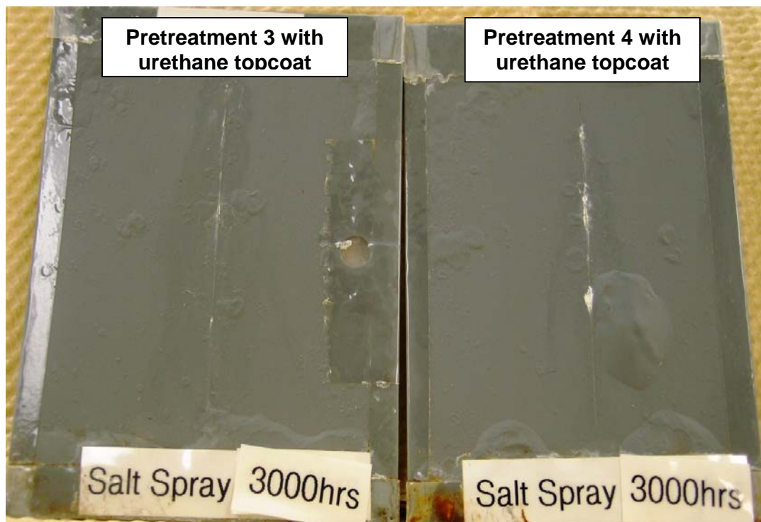
FIGURE 4 - Salt Spray Panels
