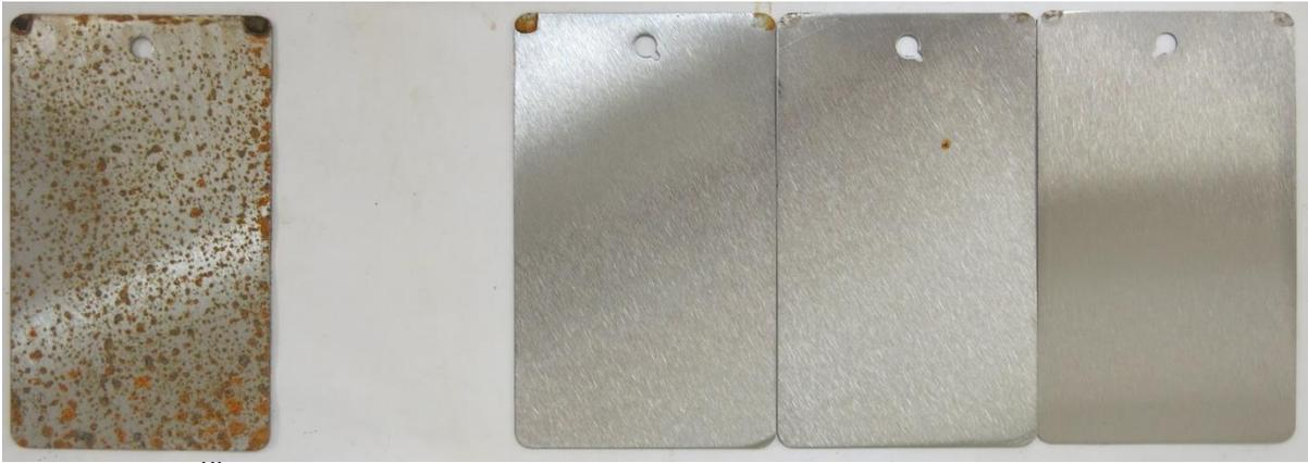
**Figure 1: ASTM<sup>(1)</sup> D-1735 test results with Product A. The control panel is pictured on the far left.**
