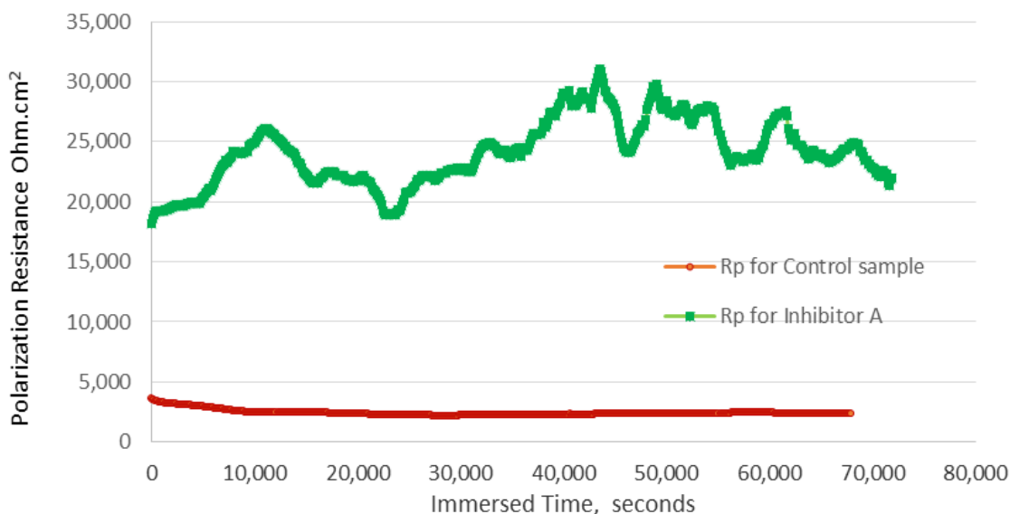
Figure 1: Polarization resistance measurements of steel rebar in 3.5% NaCl solution.
