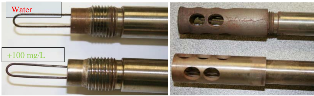
Figure 5: Comparison of corrosion ER probe surface condition of the inhibitor treated loop and control test after 2,200 hours corrosion test in hot steam/water closed loop.
