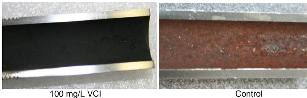
Figure 5: Comparison of steel pipe inner surface conditions of the inhibitor treated loop and control test after 2,200 hours corrosion test in hot steam/water closed loop.
