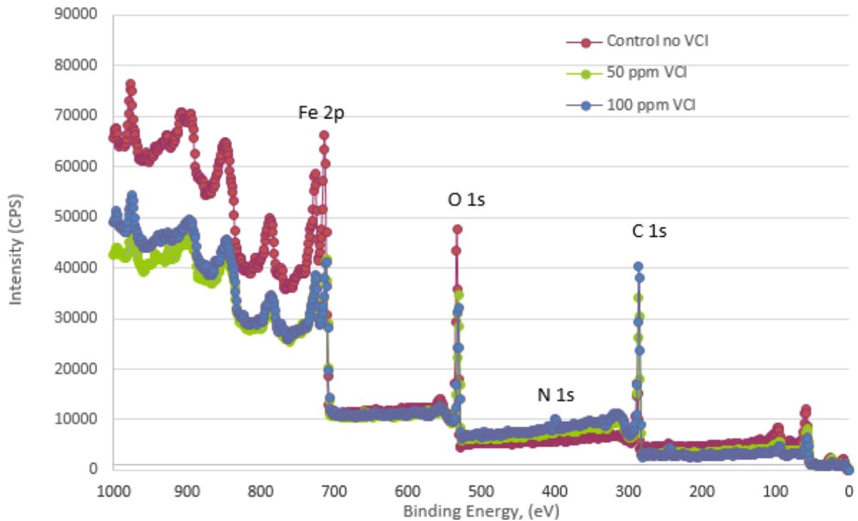
Figure 6: XPS analysis on the inner pipe surfaces after corrosion test in the hot steam loop shows more corrosion product on the control test.
