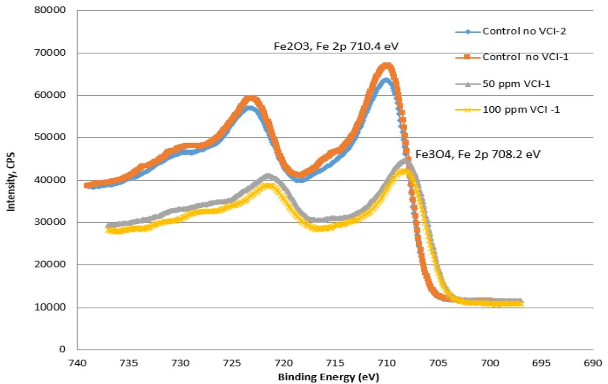
Figure 7: High Resolution XPS analysis on the inner pipe surface after corrosion test in the hot steam loop. Primary oxide seen on ID surface of non-treated pipes (control) is hematite, while magnetite is predominant oxide on ID surface of VCI treated pipes.
