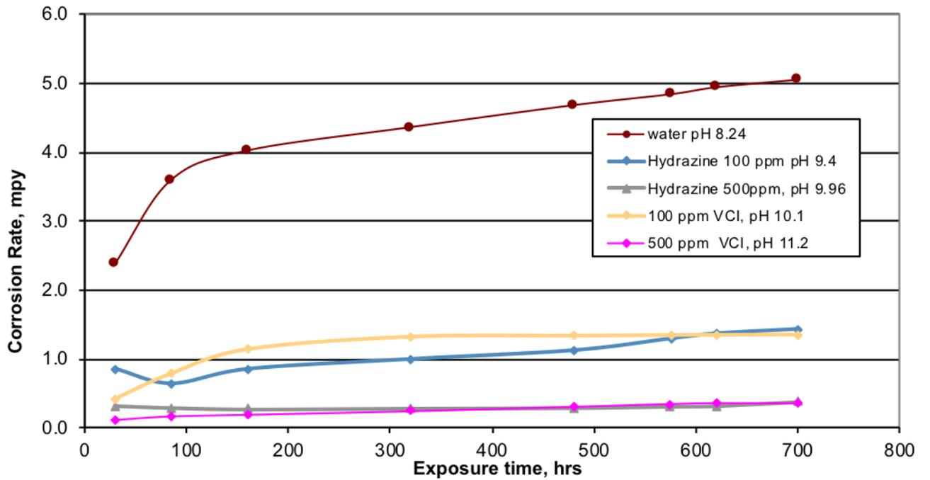
Figure 3: Corrosion behavior of steel pipes in hot water solution in 100°C when exposed to control solution, 100 and 500 mg/Kg VCI, and Hydrazine.
