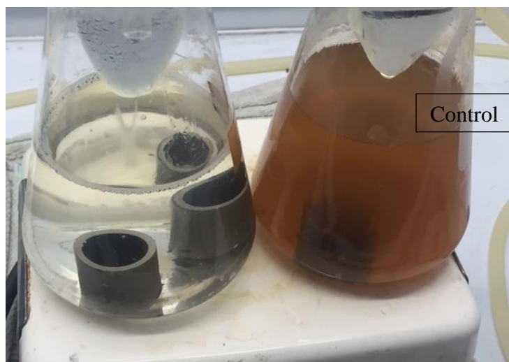
Figure 1: Corrosion set up for testing steel pipe in 200 ppm Cl - solution at boiling temperature (100 °C) with and without inhibitor.
