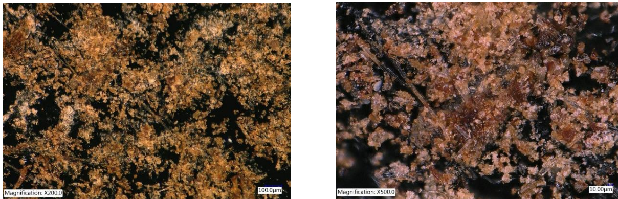
Figure 9: Pipe surface condition after CUI tests of the VCI coated pipe after five cycles of thermal cycling at 77 and 177°C, show morphology of surface deposits.
