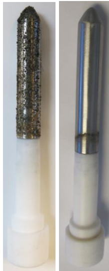
Figure 2: Contact corrosion test results per ASTM D665B. L – untreated fuel (control), R – fuel with 1.6% additive Test duration: 4h, temperature: 50°C
