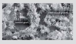
technology is a stable suspension of synthetically produced crystalline calcium silicate hydrate (CSH) nanoparticles. These nanoparticles facilitate the growth of CSH crystals between cement grains and improve the overall hydration of portland cement. The strength-enhancing property of this technology permits a reduction in the total cementitious materials content of a given concrete mixture while maintaining the compressive strength of concrete.
