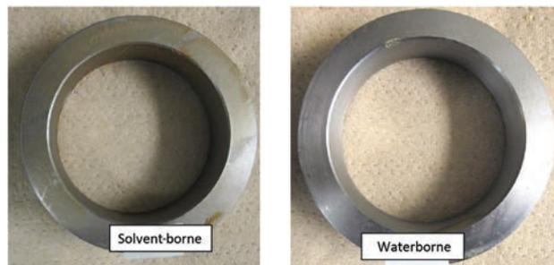
FIGURE 6 Humidity testing for solvent-borne wax coating and waterborne wax coating with VCIs (768 h).
