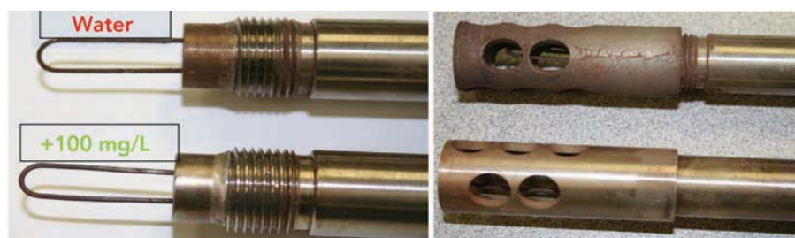
FIGURE 5 Comparison of corrosion ER probe surface condition of the inhibitor treated loop and control test after 2,200 h corrosion test in hot steam/water closed loop.
