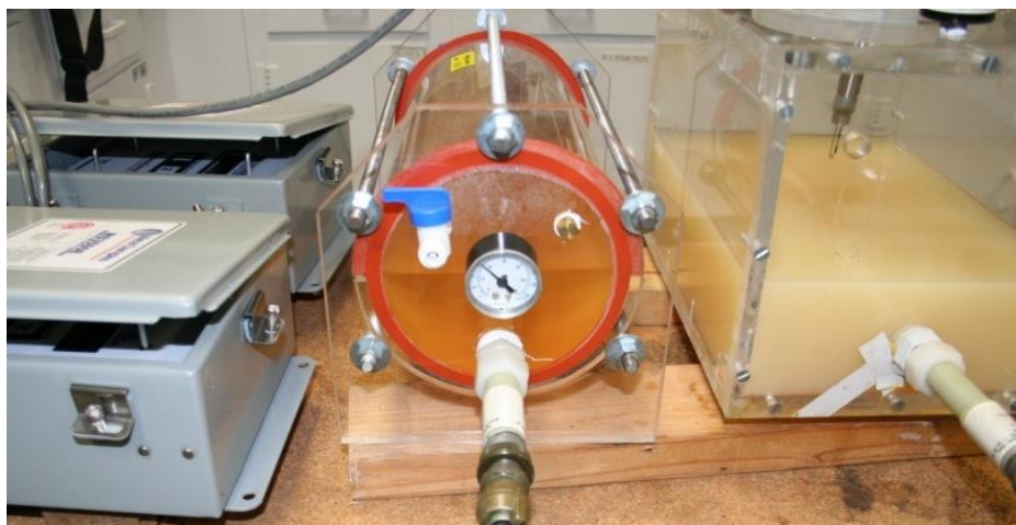
Figure 1: Test setup for corrosion test on steel LPR and ER probes using 10% VCI or nitrogen blanketing at 10 psi applied pressure.
