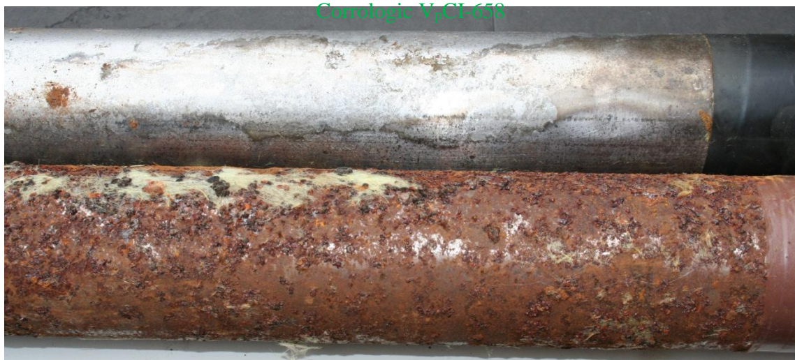
Figure 19: CCT GM protocol corrosion tests - Comparison of ER test probes and insulation/pipe interfaces after 242 days (5,800 hours); inhibitor treated pipe shows no corrosion attack, while the control sample shows red rust formation.
