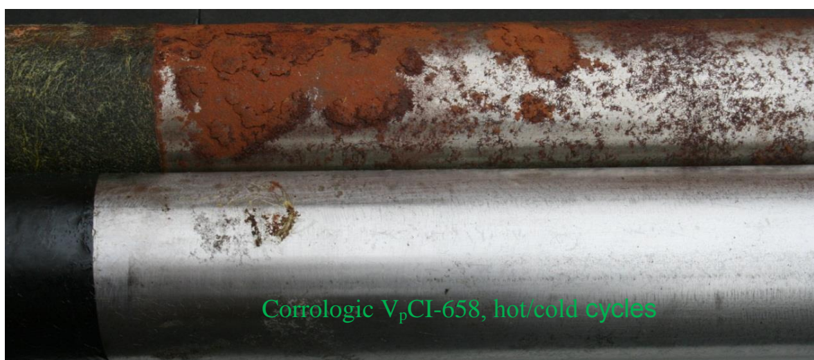
Figure 17: Hot/cold cycles - Comparison of insulation/pipe interfaces after 242 days (5,800 hours). Inhibitor treated pipe shows no corrosion attack, while the control sample shows red rust formation.
