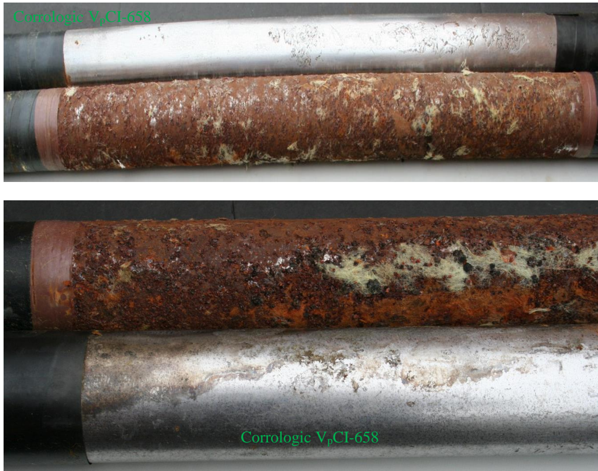
Figure 18: CCT corrosion tests - Comparison of insulation/pipe interfaces after 242 days (5,800 hours); Corrologic VpCI-658 treated pipe shows no corrosion attack, while the control sample shows red rust formation.
