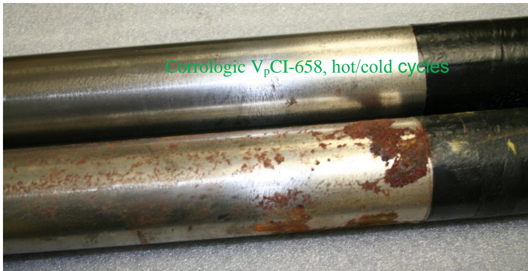
Figure 9: Comparison of surface of the insulation/pipe interfaces after 60 days (1440 hours), Corrologic V p CI-658 treated pipe shows no corrosion attack, while the control sample showed red rust formation at its interface.
