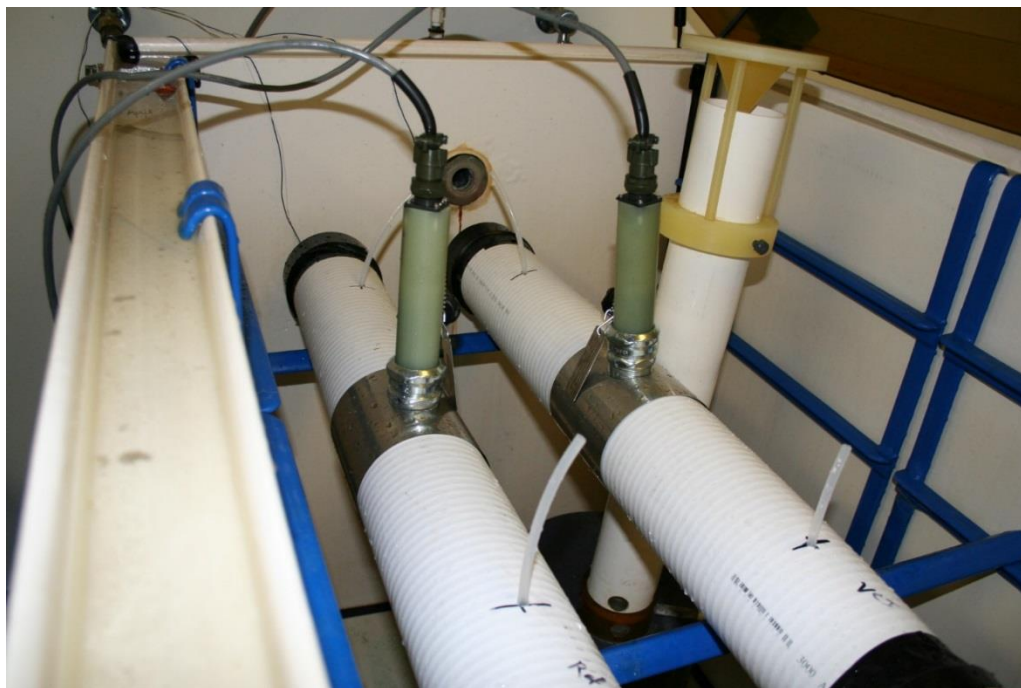
Figure 4: Assembled test samples in test chamber showing ER test probes and solution or V p CI feed tubes. Corrosion rate was recorded continuously using ER and Data collectors.
