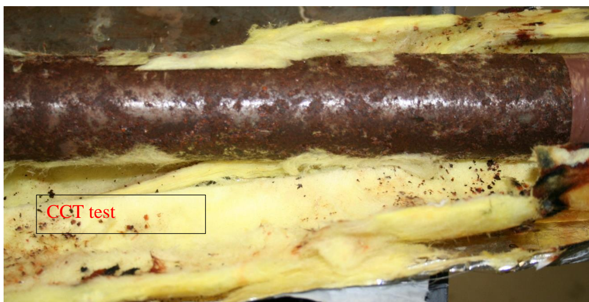
Figure 21: Photos of insulation/pipe interfaces after 242 days (5,800 hours): without Corrologic V p CI-658 treated pipe shows severe corrosion and red rust formation.
