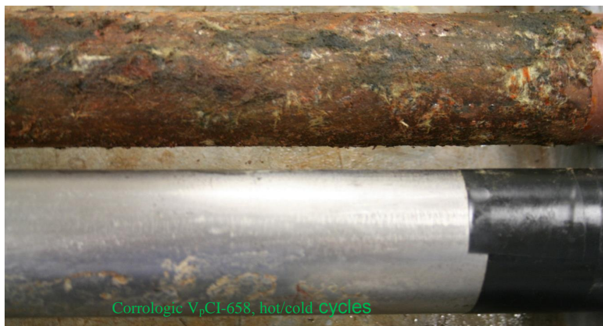
Figure 15: Comparison of insulation/pipe interfaces after 210 days (5,040 hours); inhibitor treated pipe shows no corrosion attack, while the control sample shows red rust formation.
