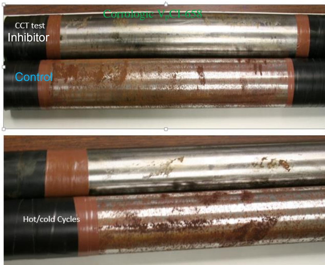
Figure 8: Corrologic V p CI-658 treated pipe shows no corrosion attack, while the control sample showed red rust formation at its interface.
