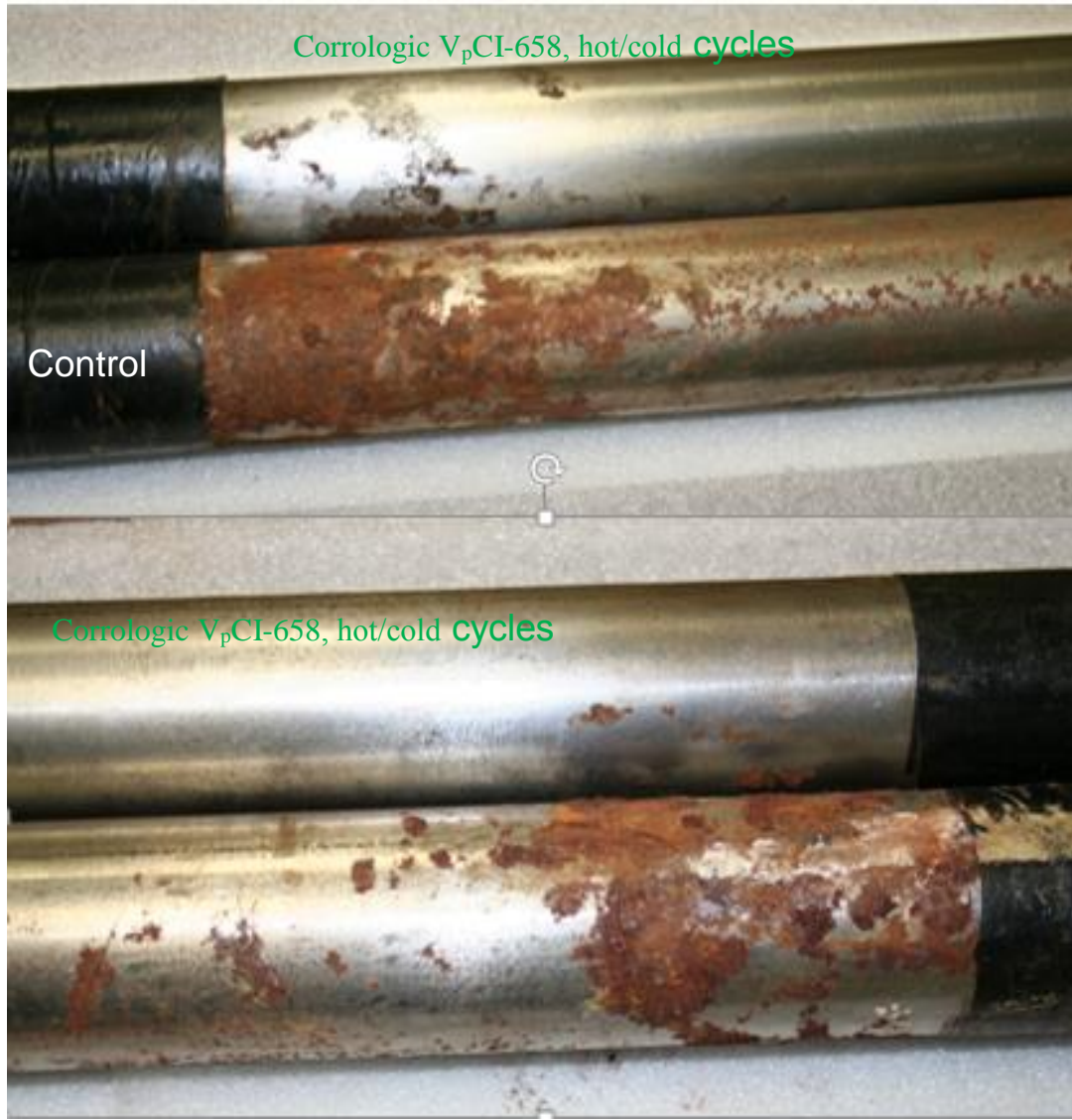
Figure 12: Comparison of surface of the insulation/pipe interfaces after 120 days (2880 hours), inhibitor treated pipe shows no corrosion attack, while the control sample showed red rust formation at its interface.
