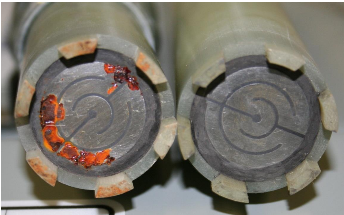
Figure 10: Comparison of electrical resistance probes used to measure the corrosion rate of the CUI samples after 60 days exposure. The control sample shows red rust formation; while sample treated with Corrologic V p CI-658 is clean and shows no corrosion residue.
