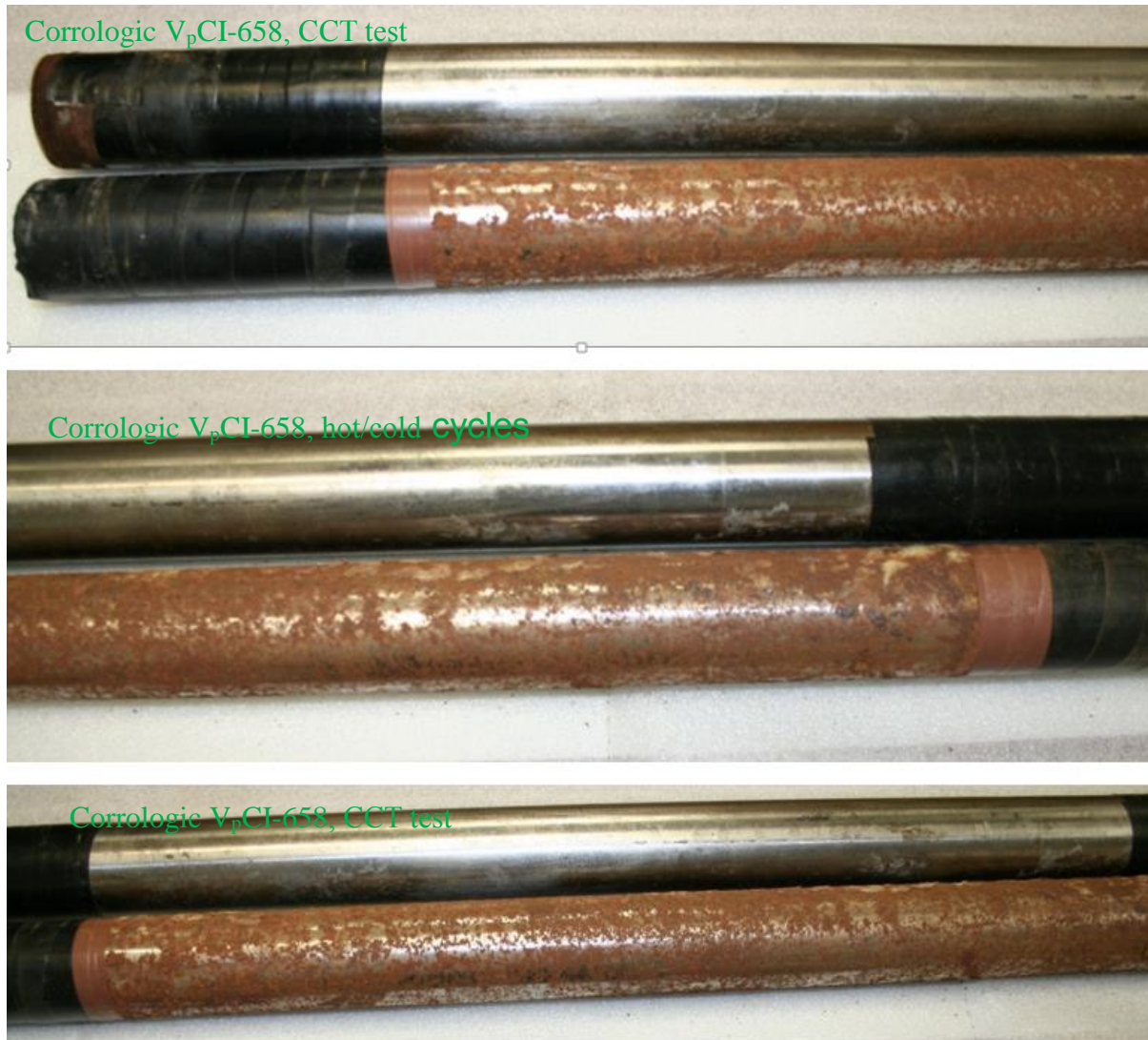
Figure 13: Comparison of surface of the insulation/pipe interfaces after 150 days (3600 hours), inhibitor treated pipe shows no corrosion attack, while the control sample showed red rust formation at its interface.
