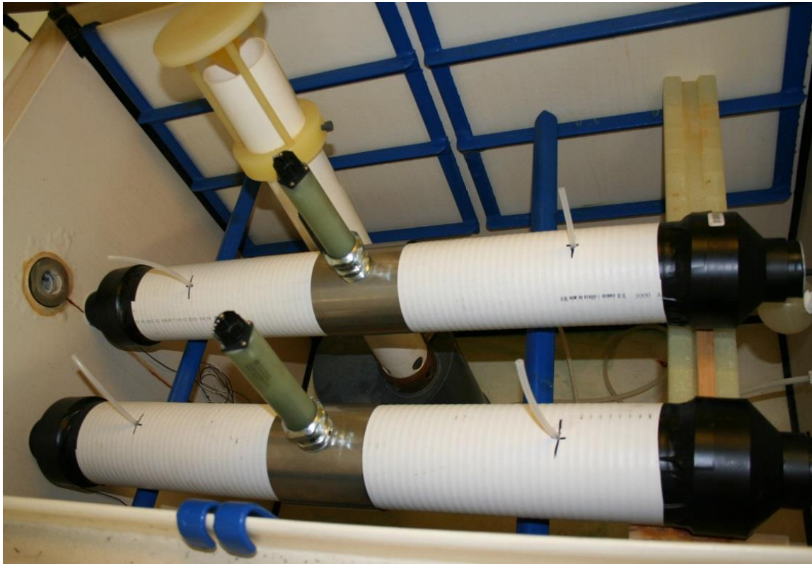
Figure 3: Assembled test samples in test chamber showing ER test probes and salt solution feed tubes. Every 48 hours, a 50 ml solution was injected at pipe/insulation interfaces.
