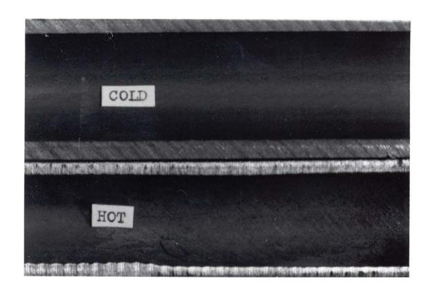
Figure 2: Typical inside surface of cold-finished tube vs. hot-finished tube.
