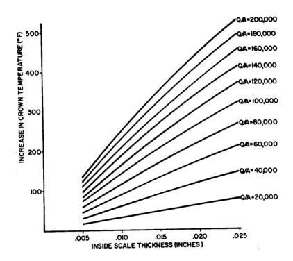
Figure 1: Temperature increase vs. scale thickness for waterwall tubes, assuming nucleate boiling.
