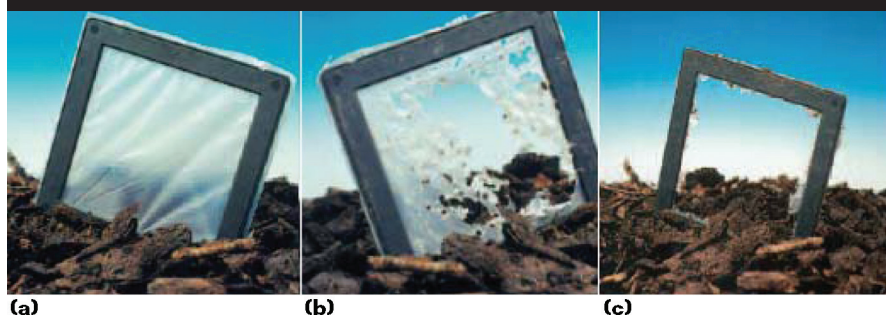
Lifecycle biodegradation process. (a) Prior to insertion into compost pile, (b) after three weeks in compost pile, (c) after six weeks in compost pile. Less than 10% of the original weight of the film is remaining after six weeks in compost pile. 10
