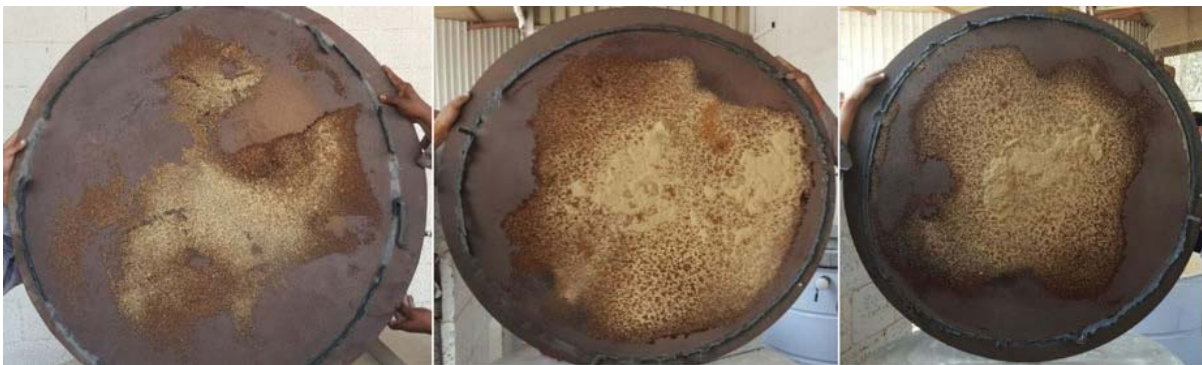
FIGURE 6. Underside steel plate of unprotected tanks at the end of pre-injection phase.
