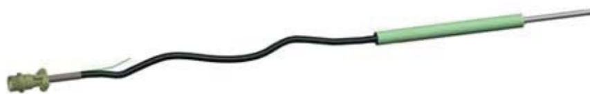
FIGURE 3. Electrical resistance probe used for the experiment.
