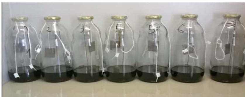
Figure 2. Experimental setup for the mass loss measurements.
