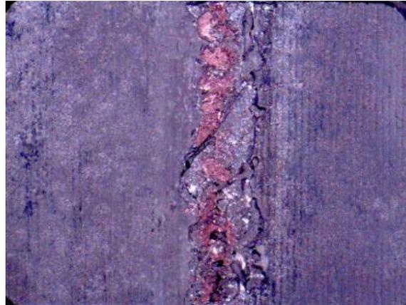
Figure 3. Traces of copper left on internal pipeline weld.
