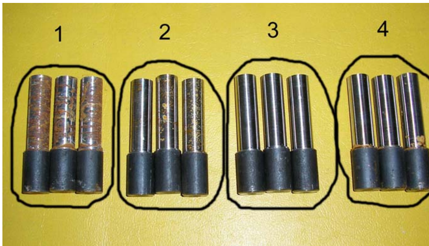
Figure 4. Appearance of samples machined with application of SHIP coolant containing inhibitor INH2 after testing 1-in salt chamber, 2-in atmospheric conditions, 3-in closed area, 4-in wet chamber
