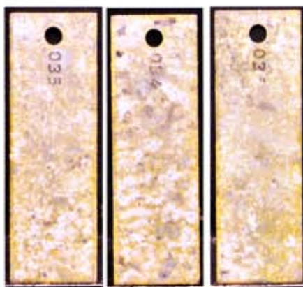
Galvanized steel coupons—control.
