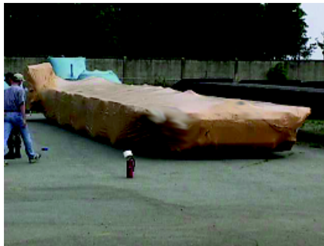
60K cargo loader with VpCI military shrink wrap.
