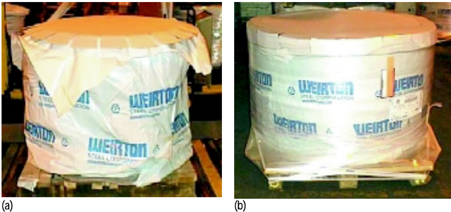
(a) A 12-t coil is shown before and after stretch wrapping.
