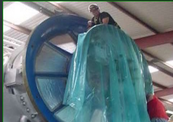
Inlet covered with VpCI®-126 Film
