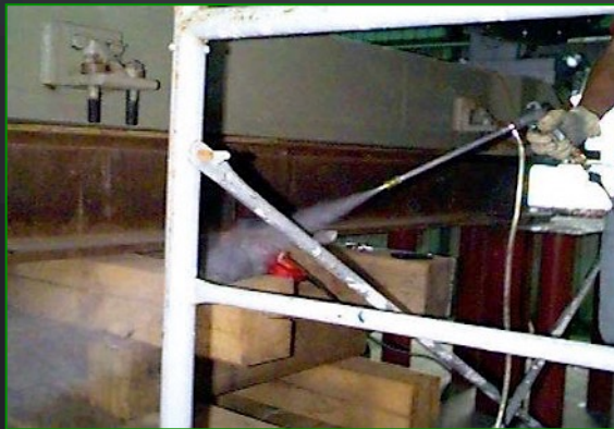
Setting discharge to a light fog
